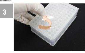
Paste the RAPID Slit Seal on the 96-well plate and make sure holes of RAPID Slit Seal are correctly positioned on each well spot.
