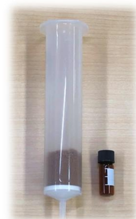
Fig. 3 60 mL reservoir (Adsorbent 10 g filled)
