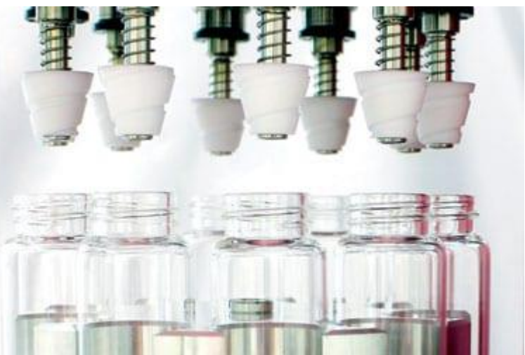
Caption: VVC technology employed by SMART evaporator (courtesy: BioChromato Inc.)
