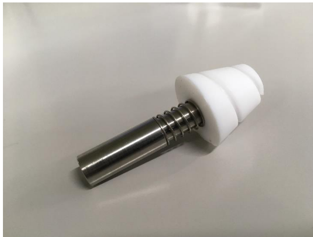
Caption: Solvent removal using VVC technology and a spiral plug adaptor for BioChromato SMART Evaporators
