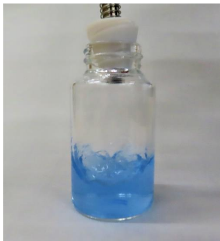
Caption: Solvent removal using VVC technology and a spiral plug adaptor for BioChromato SMART Evaporators
