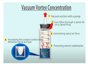
This fast and strong airflow stirs the sample very efficiently, increasing the surface of the liquid and promoting the solvent to evaporate, at the same time as sucking the evaporated solvent vapor out through the pump.
