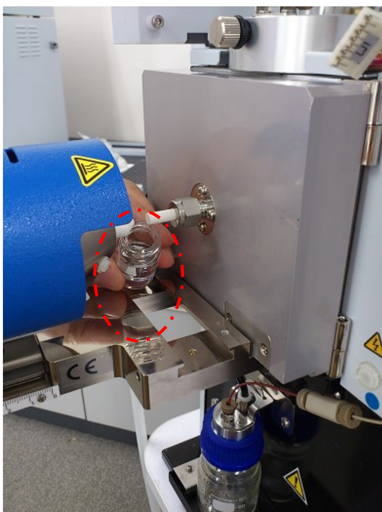
Figure 3 Standard sample (vapor) analysis by DART-MS Sample vial opened its cap was placed under DART gas flow.
